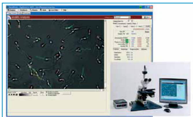
Picture 8. Components and image of the CASA system with automorphology (cytoplasmic droplet and tails are pointed with a box)
